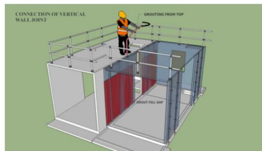
Grouting in between PPVC Modules
