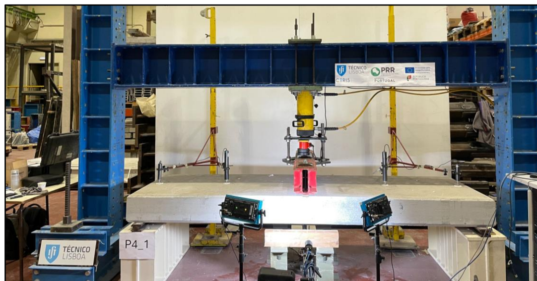
Carga centrada ( bending failure oriented )
