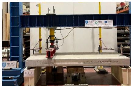
Shear failure oriented test
