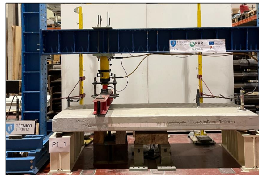
Carga excêntrica ( shear failure oriented )
