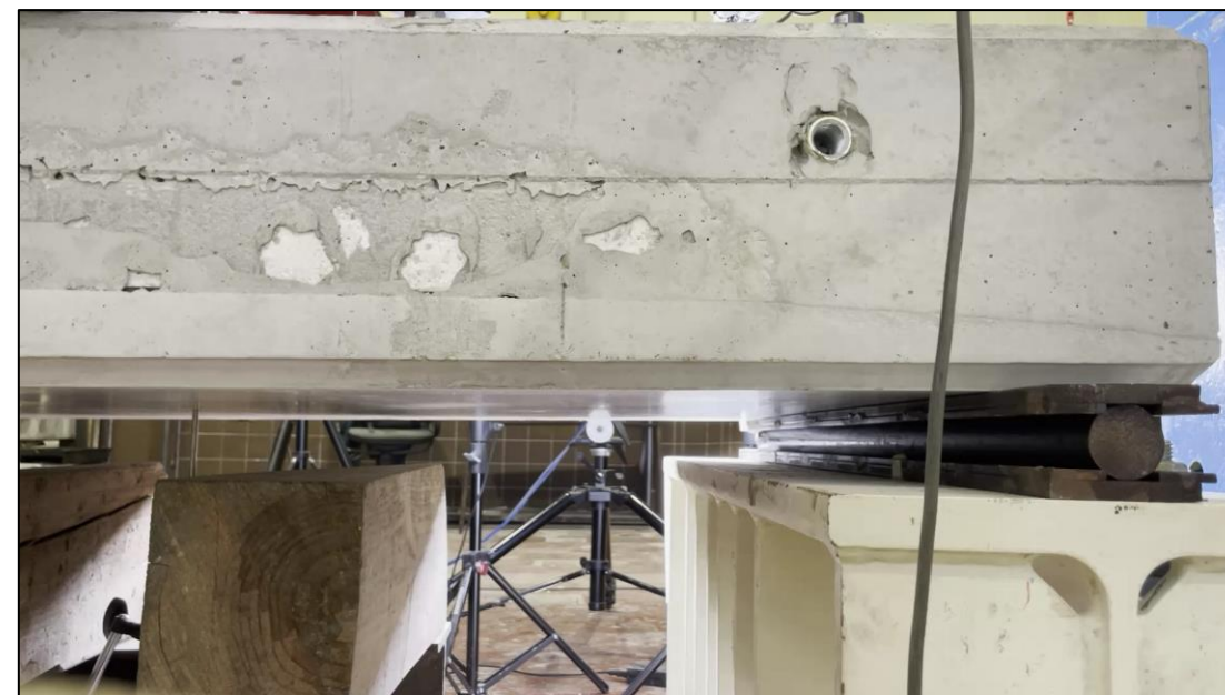
Shear failure oriented test – P1,P2,P3
