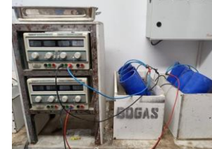
Figure 6 - Chloride Penetration Test
